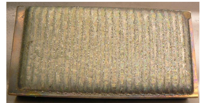
Cladding of Nickel alloy on 316L substrate
